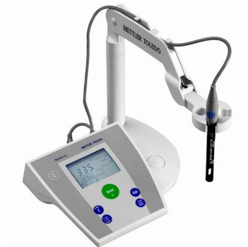
Slika 5: Konduktometar Mettler-Toledo SevenEasy S30
