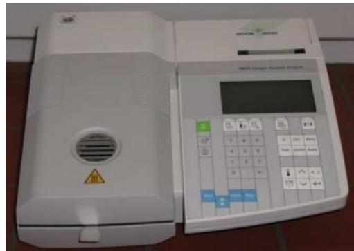
Slika 8 Analizator vlage Mettler Toledo HR 73
