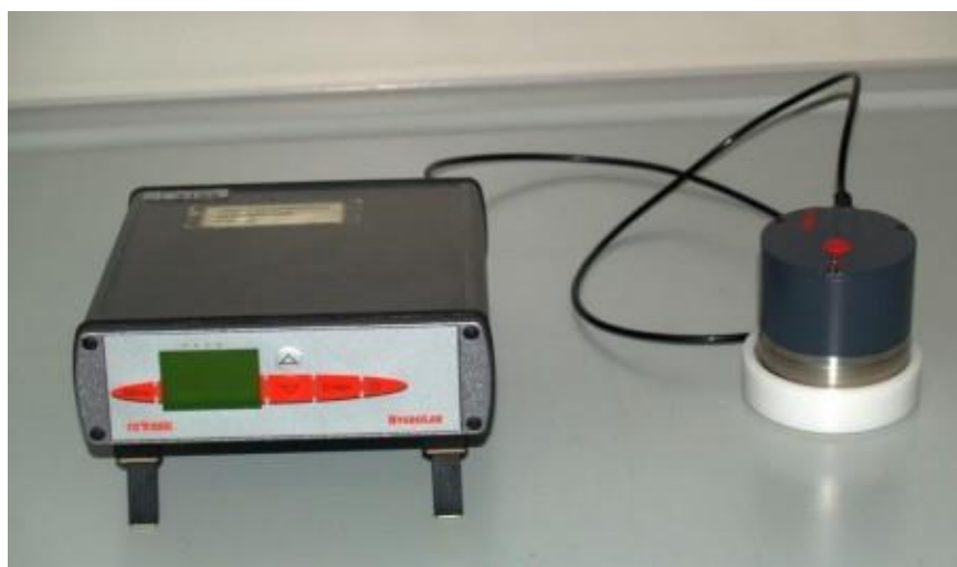
Slika 10 HygroLab 3 – Multi-channel Humidity Water Activity Analyser
