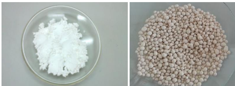
Fig. 1. Zeolites: powdered zeolite (ZAP) and granulated (ZAG)
