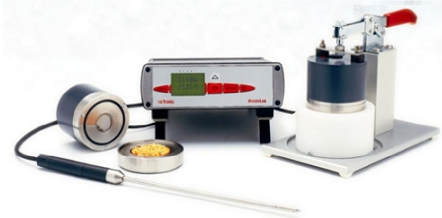
Slika 11. Rotronic - HygroLab 3 – Multi-channel Humidity Water Activity Analyser
