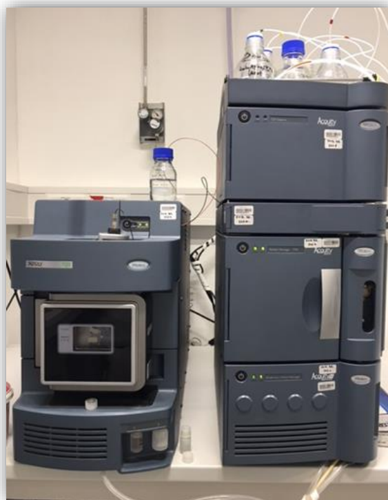
Slika 19 UPLC-MS/MS instrument Acquity H-class-Xevo TQD MS (Waters, SAD)
