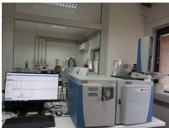
Slika 2. Plinski kromatograf s masenim spektrometrom (GC-MS/MS) Figure 2. Gas chromatograph with mass spectrometer (GC-MS/MS)
