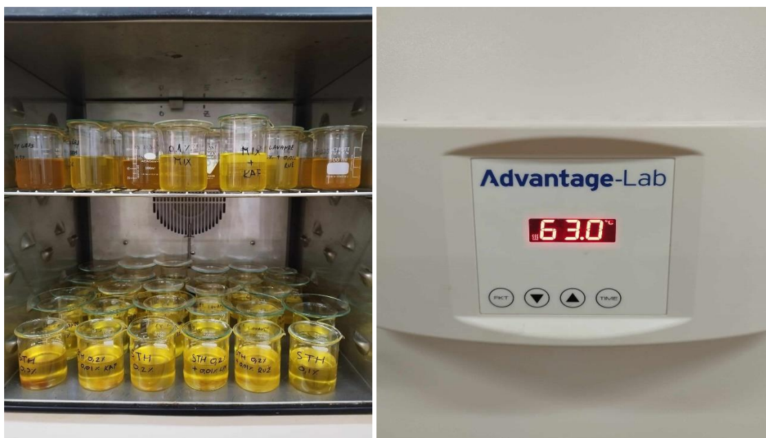
Slika 27 Schaal oven test
