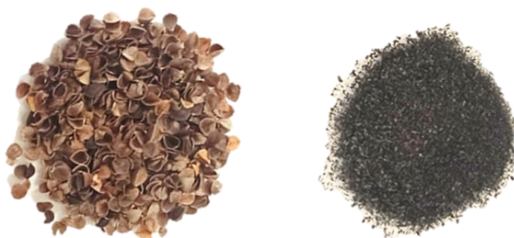
Figure 1. Physical appearance of unmodified buckwheat hulls alongside biochar derived from buckwheat hulls
