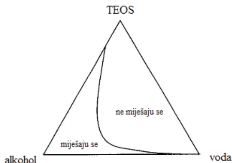
Slika 1. Fazni dijagram sustava TEOS – alkohol – voda Fig.1. Phase diagram of system TEOS – alcohol – water
