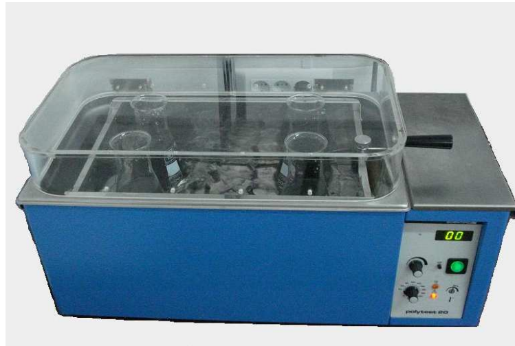
Slika 18. Termostatska tresilica Polytest 20, Bioblock Scientific.
