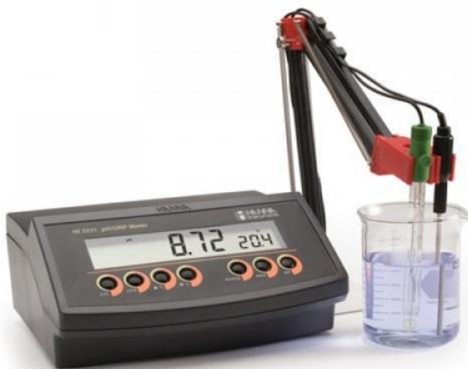
Slika 6. pH – metar (Hanna Instruments 2211 pH/ORP Meter).
