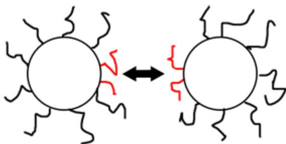
Slika 3 Sterička stabilizacija ([http://www.wikiwand.com/en/Polyelectrolyte\\_adsorption](http://www.wikiwand.com/en/Polyelectrolyte_adsorption))
