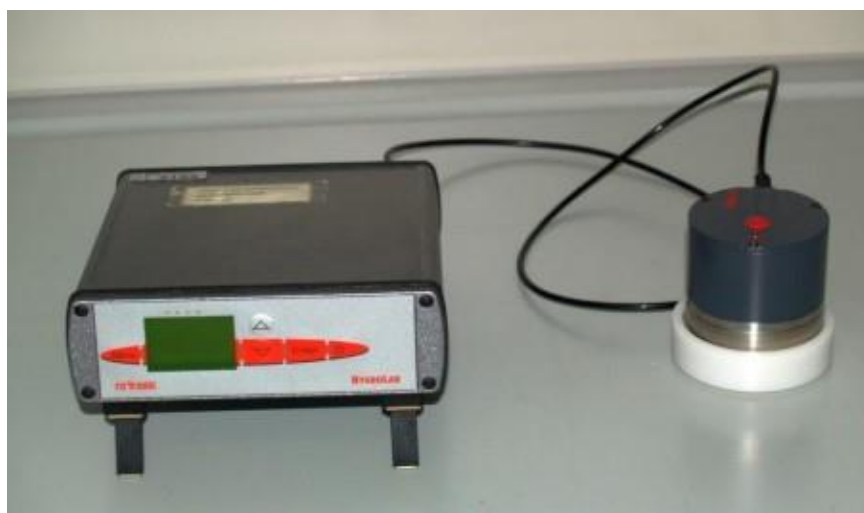
Slika 10 HygroLab 3 – Multi-channel Humidity Water Activity Analyser
