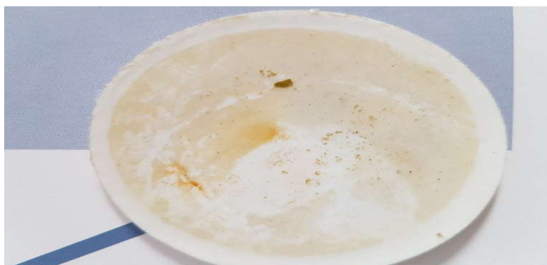
Fig. 8. Deposits on the membrane surface after filtration
