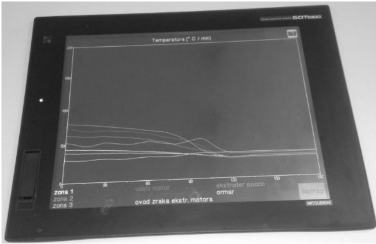
Figure 3. Temperature parameters of production of bread chips (at the facility)
