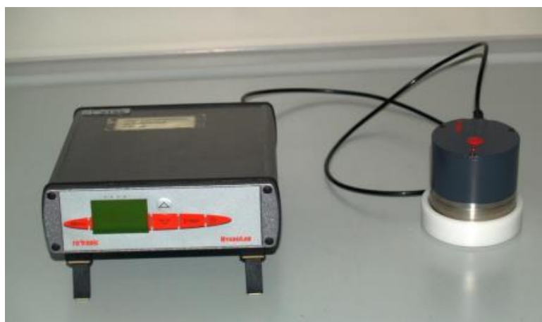
Slika 7. Rotronic - HygroLab 3 – Multi-channel Humidity Water Activity Analyser
