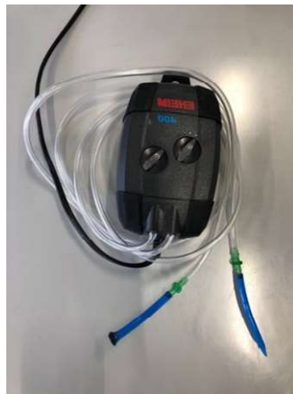
Figure 19 Electric pump EHEIM 400 for aeration of wastewater
