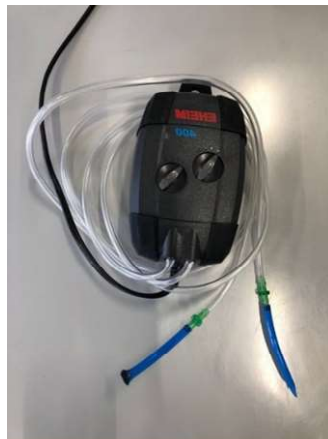
Figure 19 Electric pump EHEIM 400 for aeration of wastewater
