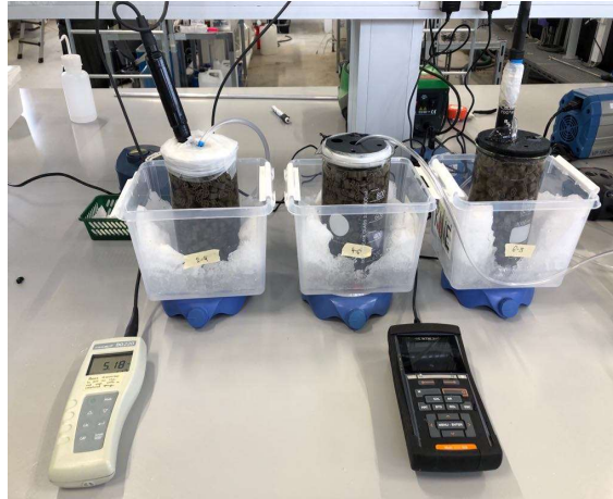
Figure 20 Three bioreactors with sample and carriers
