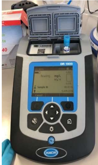
Figure 13 Spectrophotometer Hach DR 1900 used for measuring concentrations of measured parameters
