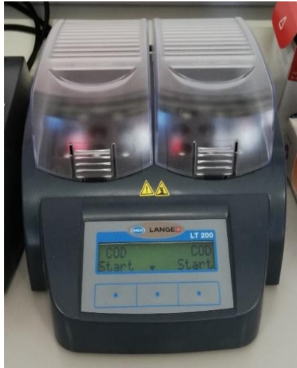
Figure 7 Thermostat Hach LT 200
