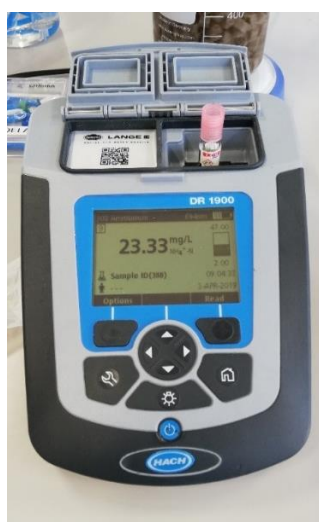
Figure 6 Spectrophotometer Hach DR 1900 used for wastewater analysis
