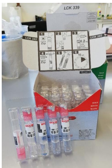
Figure 5 Hach Dr. Lange cuvette test LCK 342 Nitrite
