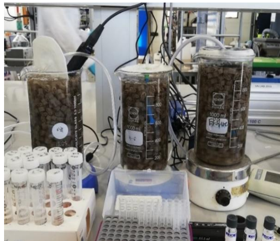
Figure 13 Mixed bioreactors of the same content into which different oxygen concentrations are blown
