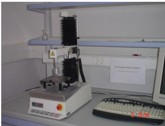
Slika 7 TA.XT2 Plus Texture Analyser (Tanasković, 2014)
