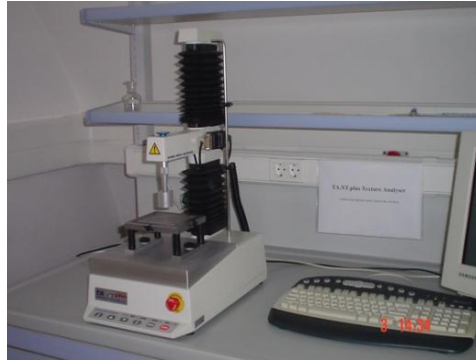
Slika 7 TA.XT2 Plus Texture Analyser
