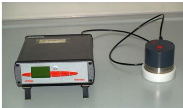
Slika 19 Rotronic – HygroLab 3 – Multi – channel Humidity Water Activity Analyser
