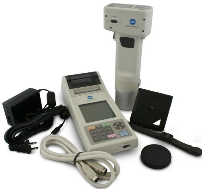
**Slika 8.** Kolorimetar Konica Minolta CR-400 (Web 8)
