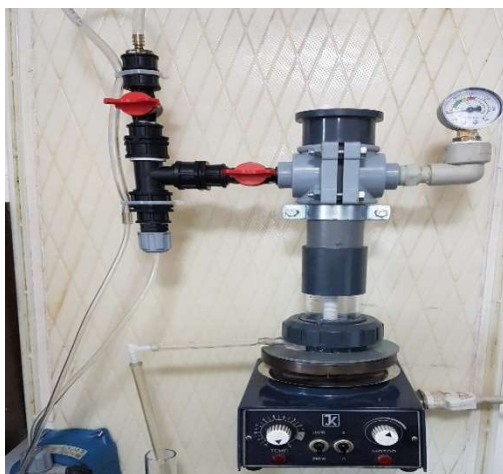
Fig. 1. Dead end filtration system
