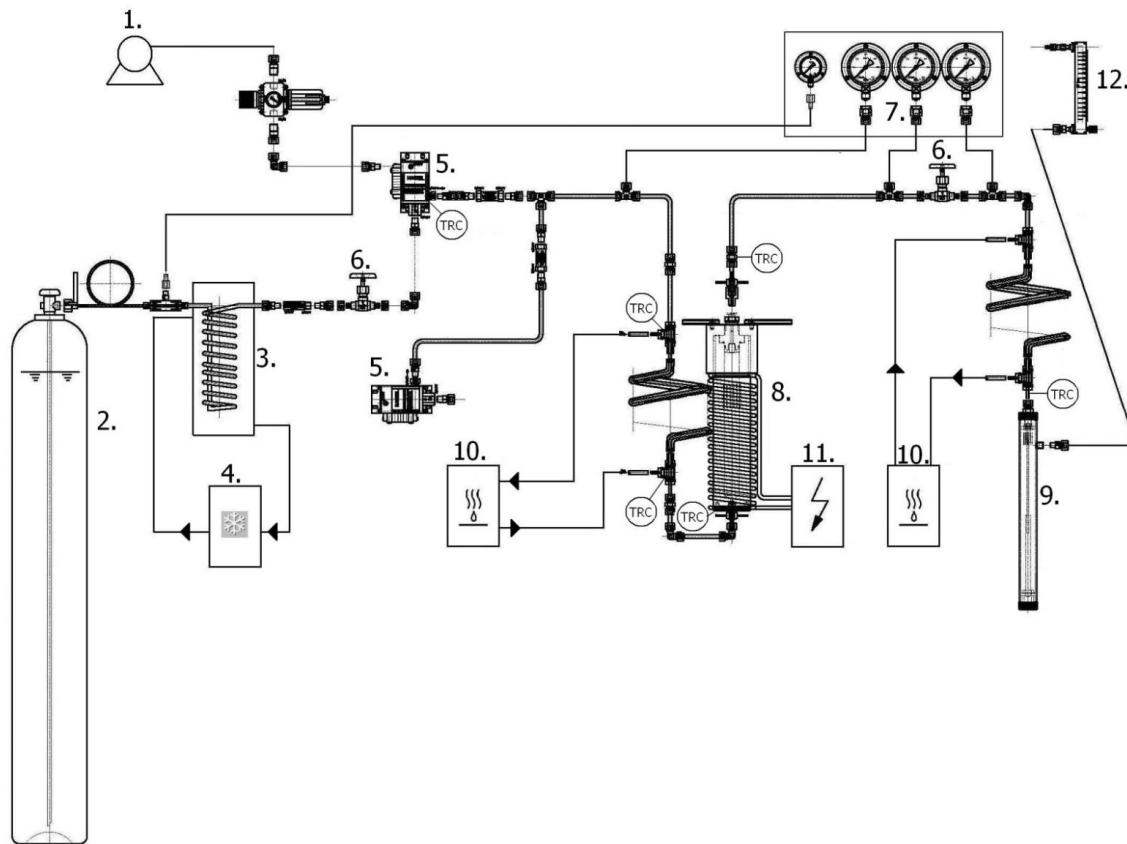
**Fig. 1.** Experimental set-up of supercritical fluid extraction system
