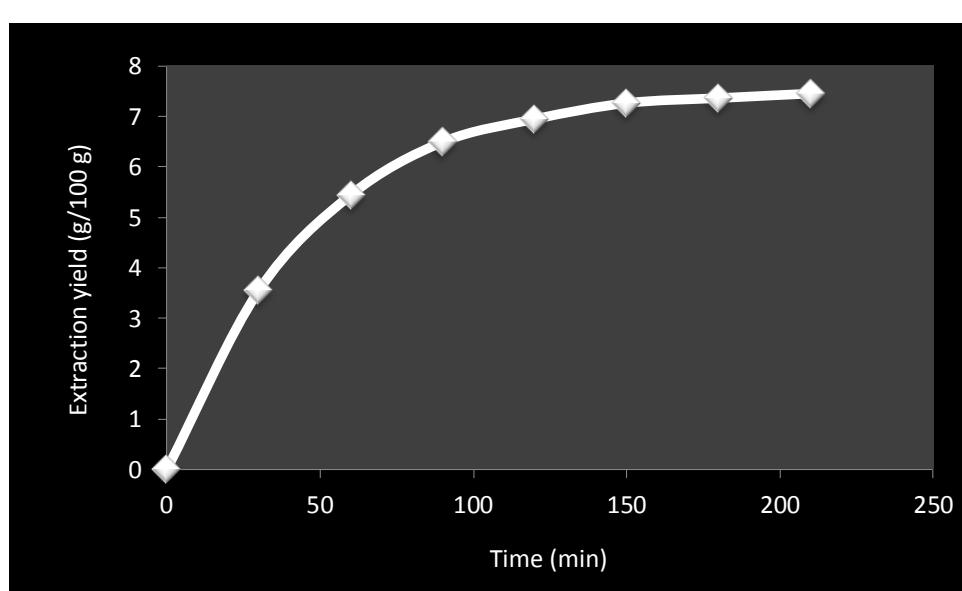
**Fig. 3.** Extraction of cake residual oil with supercritical CO<sub>2</sub>
