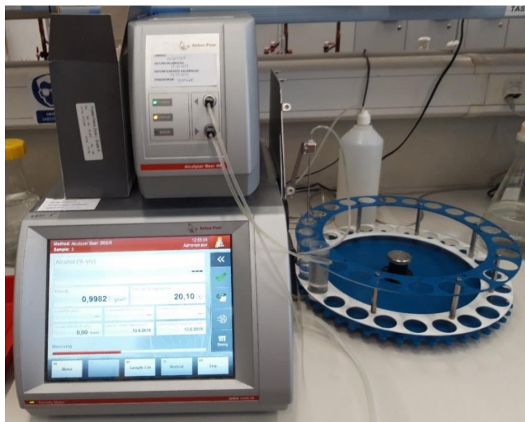
Slika 5 Analizator piva (Alcolyzer Beer Analyzing System, Anton Paar, Austrija)
