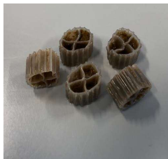
Figure 8 Used plastic carriers with attached biomass
