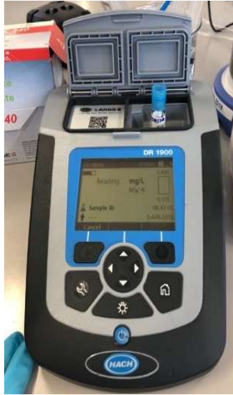
Figure 13 Spectrophotometer Hach DR 1900 used for measuring concentrations of measured parameters
