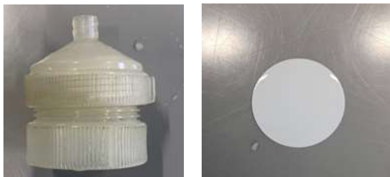
Figure 11 Filter and cellulose and nitrate (0.45 \mu\text{m} ) filter paper
