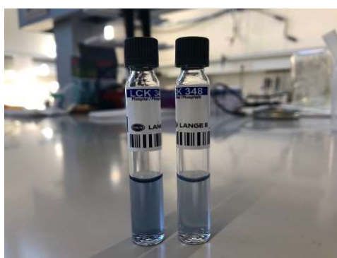
Figure 12 Hach Dr. Lange cuvette tests for Phosphorus total / Phosphate ortho LCK 348
