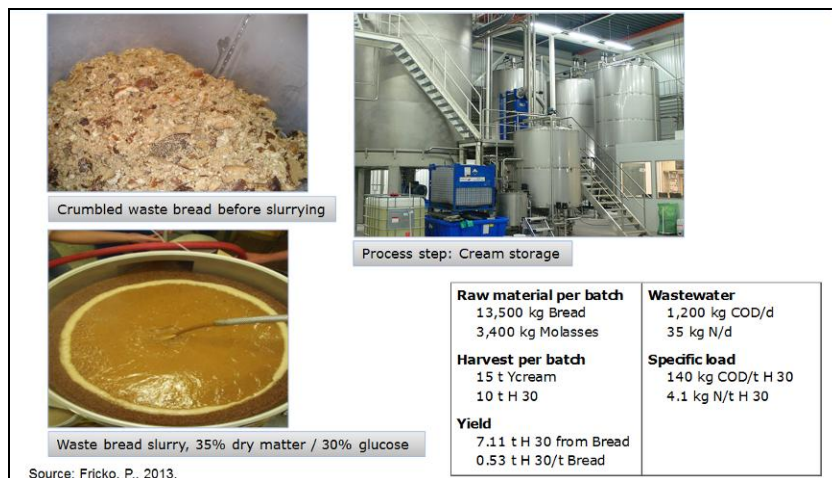
Figure 7. Production of baker's yeast by applying saccharified waste bread in combination with molasses as substrates
