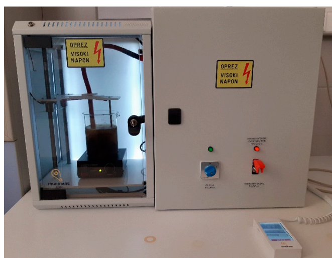
Figure 1. High voltage electrical discharge device.
