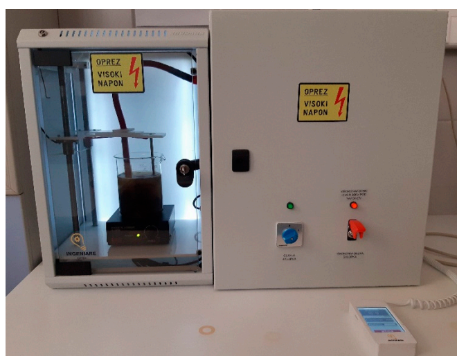
Figure 1. High voltage electrical discharge device.
