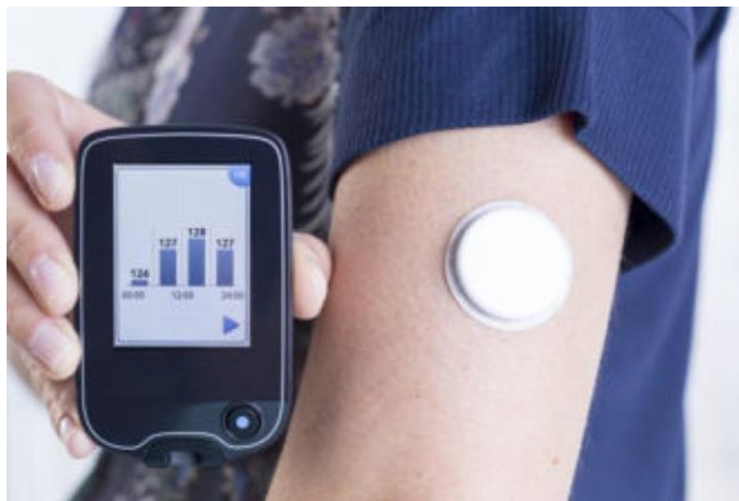
Slika 8 FreeStyle Libre Flash Glucose Monitoring System (Kleinman, 2019.)
