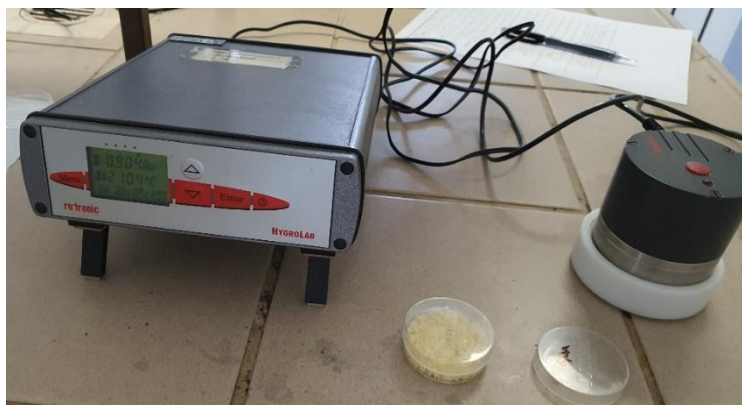
Slika 7 Rotronic HygroLab 3 (Rotronic AG, Bassersdorf, Switzerland)
