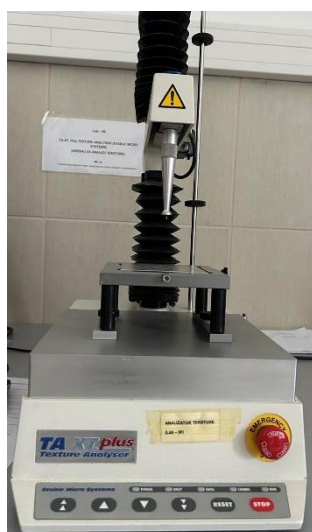
Slika 8 Universal TA-XT2i texture analyzer
