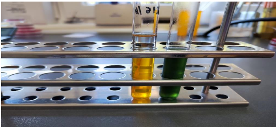
Figure 2. Oxidative-Fermentation Test (O/F Test): Positive: Yellow color/Negative: Green color
