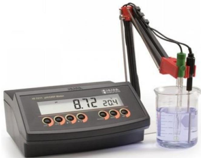
Slika 6. pH – metar (Hanna Instruments 2211 pH/ORP Meter).
